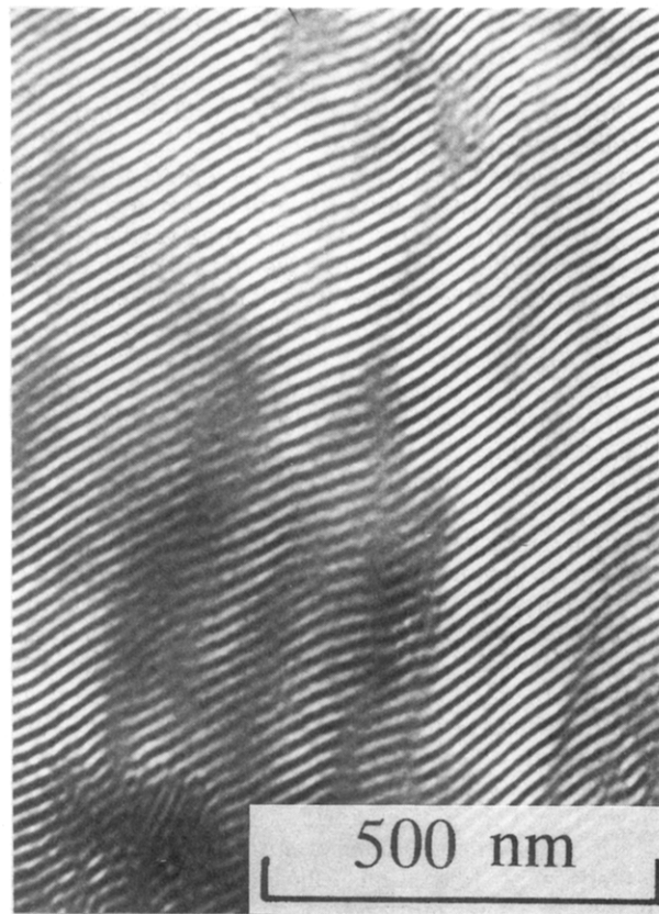
Figure 9. Electron micrograph of the 120-min annealed specimen (annealed at 150 °C).
